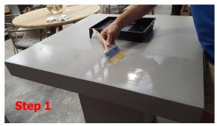
Apply a thin coat of Fila W68 to a section of the furniture. Allow sealer to penetrate for 5 minutes
