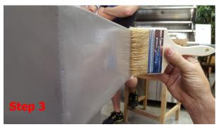
Seal edges of table and remove residues after 5 minutes with cloth as per previous steps.
