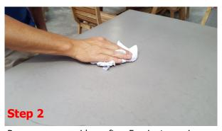
Remove any residue after 5 minutes using a clean white cloth in a circular motion. Continue sealing table in sections removing residues as per previous steps.
